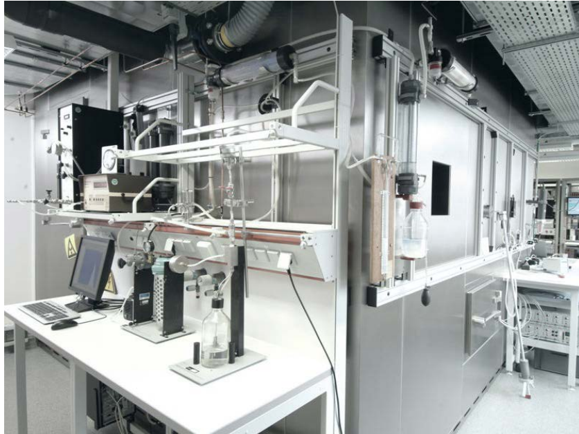
Part of the Calibration Service Laboratory with PAEC chamber for calibration of devices measuring radon progenies ( 30 \text{ m}^3 )
